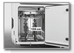
Patented Pedelec scooter garage, loading height extension up to 124 cm in conjunction with push-in and transport system
