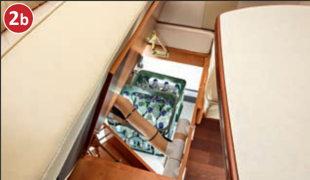
Easy removal of the storage compartment contents from the inside via the lift-up seat bench cover of the L-shaped lounge seating area with patented fitting
