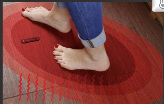
Carthago underfloor heating effect Numerous hot air outlets and heat circulation channels in the double floor ensure that the heat is evenly distributed. This heat accumulation radiates upwards towards the floor of the living area and gives it a pleasant warmth. You always have warm feet in a Carthago.
