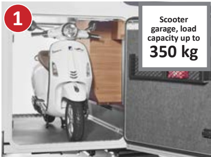
Scooter garage with interior height of up to 120 cm thanks to deep lowering, with access from both sides via two large scooter garage doors at the driver and passenger sides
