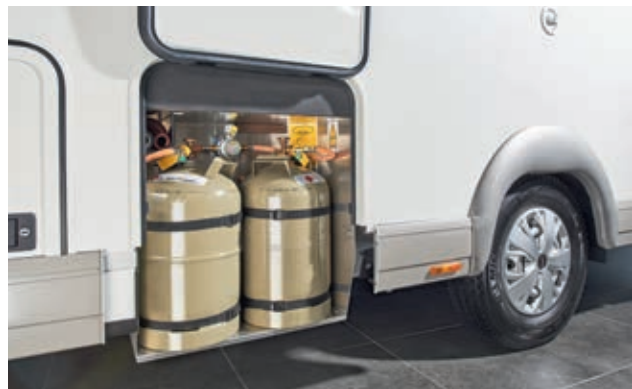
"easy change" gas bottle compartment, extra-low for convenient bottle changing
