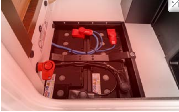
Heated battery centre with main power switch. Standard: Gel batteries 2 x 80 Ah, positioned in exterior storage space on passenger side for easy access, optional Lithium ion battery, 90 Ah including battery computer and separate touch display
