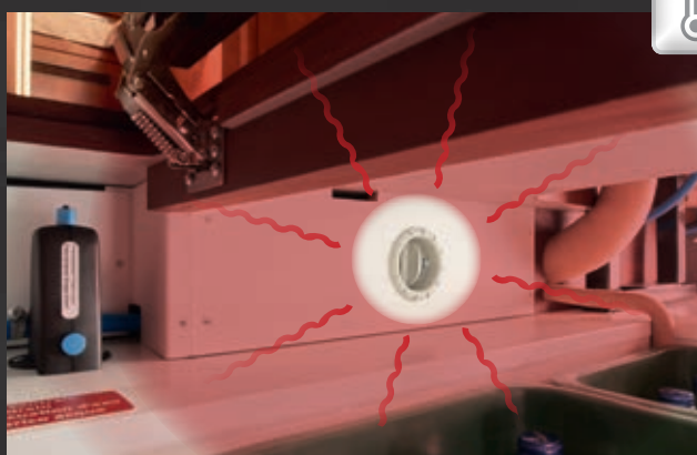
Truma Combi 6 warm air storage heating system with numerous warm air outlets throughout the double floor, the living area, the roller garage and the cold-sensitive door entrances.
