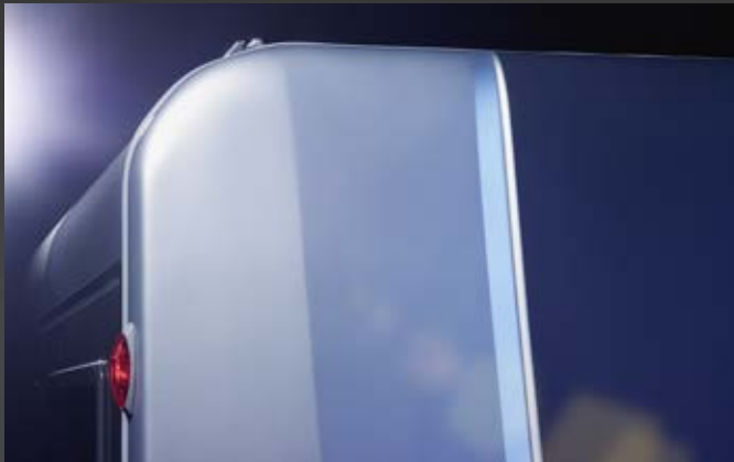
The Carthago curved roof: a Carthago awakens emotions because of its independent and elegant design such as the curved roof that is typical of the brand. It also increases the torsion resistance of the body, and there is less susceptibility to side wind. The perfect combination of design and practicality!
