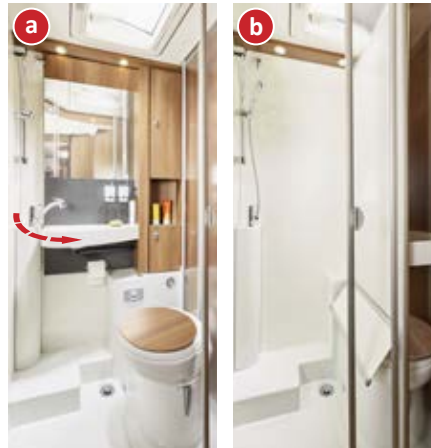
Vario swivelling washroom: Washroom and toilet a or shower room b thanks to wash stand mirrored wall that can be swivelled away
