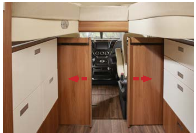
beneath the drop-down bed to prevent the ingress of cold from the driver's cabin in the sleeping configuration
