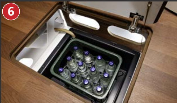
Living area floor hatch with double floor storage box (42 cm usable depth) in heated double floor
