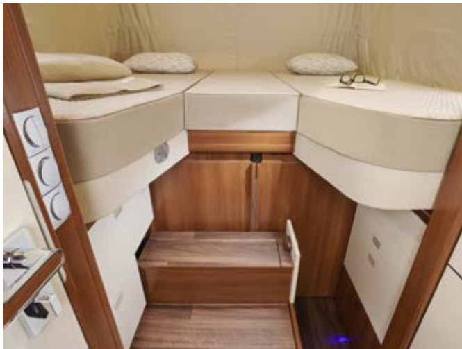
Electrically lowerable lengthways single beds with pull-out access steps and sliding doors to prevent the ingress of cold
