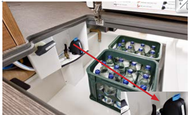
Central water drain and water tanks in the frost-proof double floor basement; can also be operated from the outside through the XL habitation door
